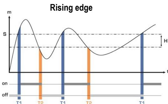
Measurement ( $m$ ) > Threshold ( $T$ ) during time-delay  $T1 \rightarrow$  Alarm activation.
