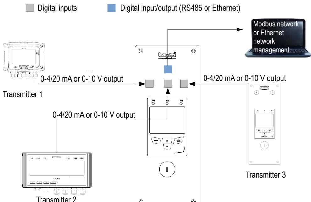
The ATE310 recovers the transmitted data by the transmitters 1, 2 and 3 via the analog inputs and displays them. The ATE310 can also transmit them to a computer via the RS485 or Ethernet connection.
