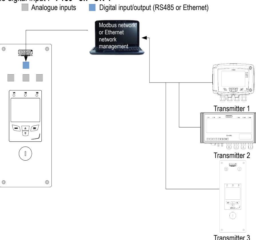
The ATE310 recovers the transmitted data by the transmitters 1, 2 and 3 via the digital input in RS485 or Ethernet and displays them.
