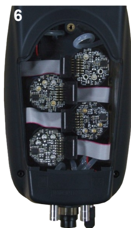
Connection of the sensor ribbon cable
