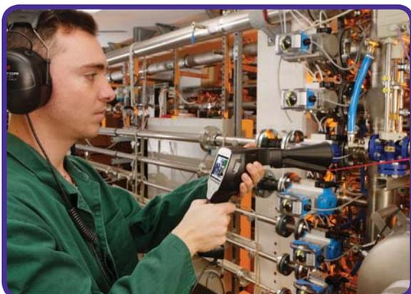
The noise-proof headset enables the leak detection also in EXTREMELY loud ambient. The ambient noise will be faded out, the leakage (inaudible ultrasonic sound) will be transformed to an audible signal. The laser grants an exact locating.
