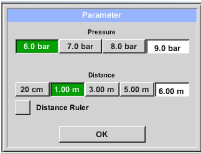
The pressure entry can be made by selecting one of the 3 predefined values or via the text field. Max. Permissible pressure value is 10bar. In case of higher pressures, please insert 10bar)
