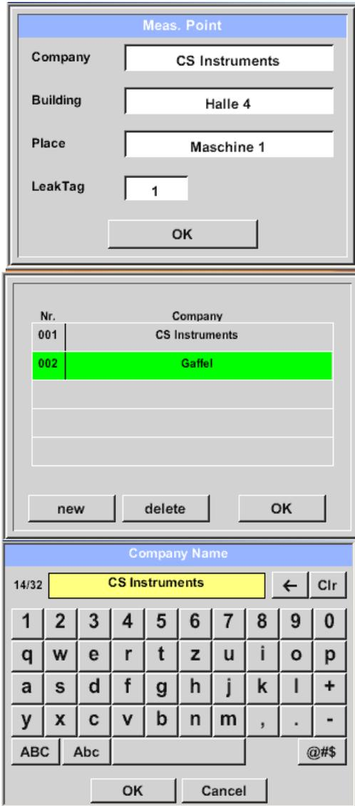
All information about the measuring point can be changed by selecting the corresponding text field or the stored measuring points can be loaded from the internal database.
