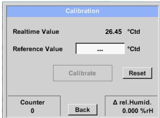
Here, a one-point calibration can be performed.
