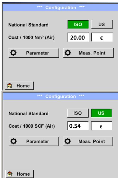
By selecting the national standard of „**ISO**“ or „**US**“ you can store your production cost for „**1000 Nm<sup>3</sup>**“ or „**1000 SCF**“. These inputs are used as the basis for the cost calculation.
