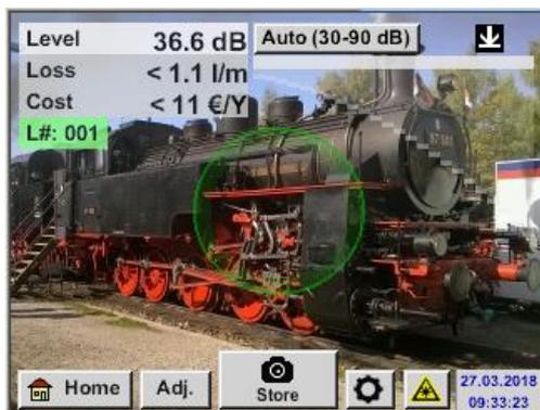
For this adjustment, the LD 500 should point to a quiet point and the adjustment should be started by pressing the „**Automatic**“ button.
