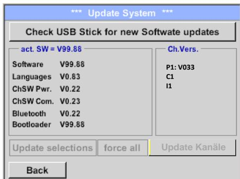
If after pressing the button *“Check USB Stick for new Software updates”* the following messages appear in the window, is the LD 500 is not properly connected to the USB flash drive or there are no files available.
