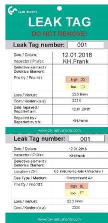
If necessary, fill out the LeakTag-form and attach it to the measuring location.
