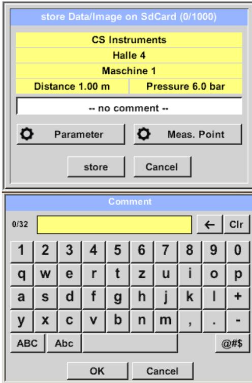
In addition to the details of the measuring point with company, building and location, it is possible to enter a comment (up to 32 characters).
