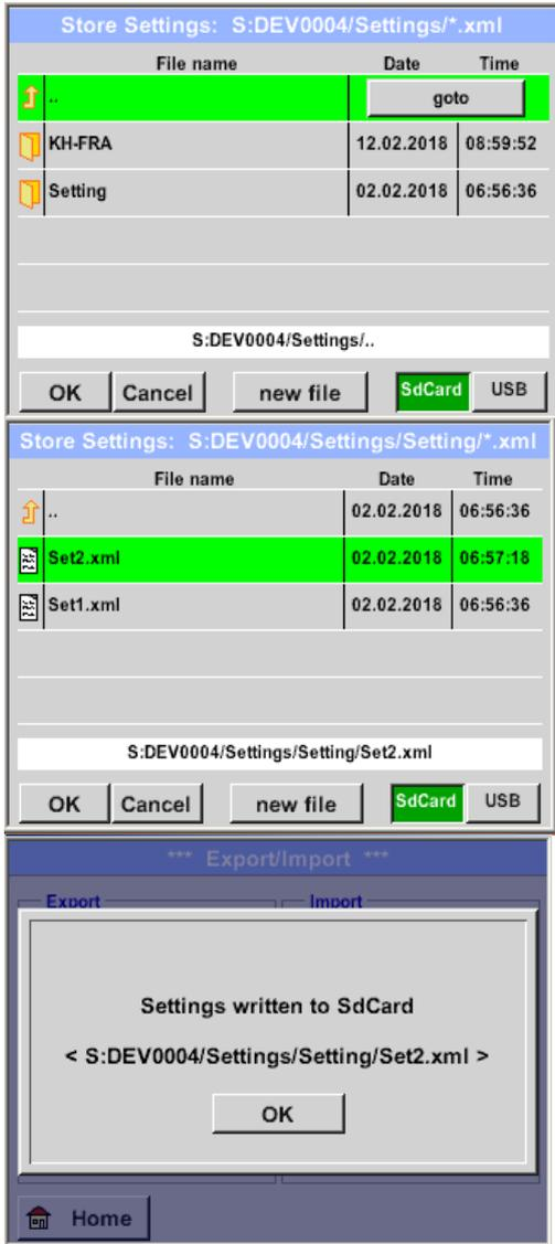
Sequence of directory and file selection is analogous to file export. Selection of internal SD card with activation of key „**SdCard**“ or on USB stick with key „**USB**“.
