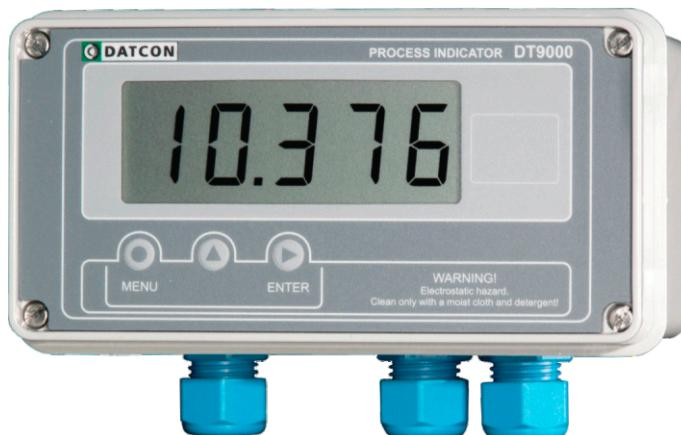
The **DT9000, DT9002 Intrinsically Safe Process Indicators** enable linear process variables to be displayed in engineering units in even the most hazardous plant areas (zone 1, zone 2). Two isolated outputs are available with different operating modes for limit signaling or for simple control purposes. Both indicators are loop-powered from 4-20 mA signals, dropping less than 2 V at 20 mA.
