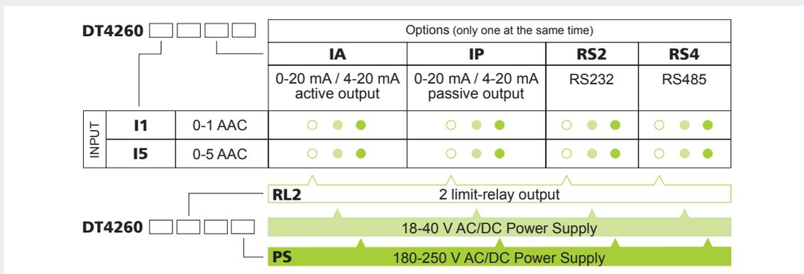
The DT4260 ... AC Current Meter enable 0-1 AAC / 0-5 AAC current ranges to be displayed on the control panel. Large 5 digit, 14.2 mm height LED display make process value easily visible at a distance.
