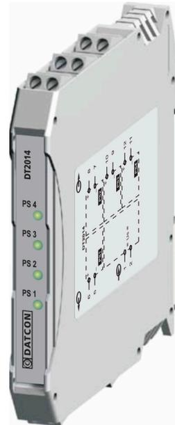
The **DT2014 Four-channel Power Supply** is designed primarily to supply power for two-wire 4-20 mA transmitters. The unit provide four galvanically isolated 22 VDC, 25 mA stabilized outputs. The outputs are overcurrent-protected with limiter characteristics.
