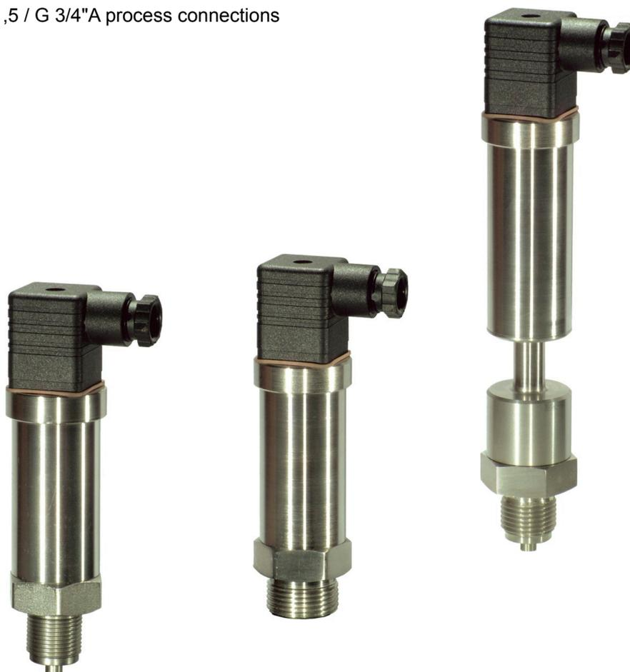
The **DT7200 ...Intrinsically safe pressure transmitters** provide a 4-20 mA current signal in proportional to the pressure connected to their input. The transmitters are intrinsically safe devices, and they can be operated in a potentially explosive environment falling into the category Zone 0 and Zone 1.
