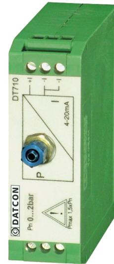
The **DT710 Pressure-current converters** provide 4-20 mA current signals proportional to the pressure connected to the devices input. The transmitters are available with 11 different measurement ranges.
