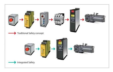
37 can be used as "safe coast" for this purpose – the stop function satisfies stop category 0 EN 60204-1. Expensive and bulky external components can be omitted, wiring simplified, and down-time minimised with
