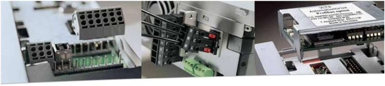
To disconnect wires, simply unplug the terminal blocks.
